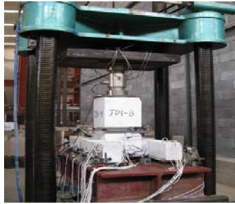
Fig. 3 Load and displacement measurement
